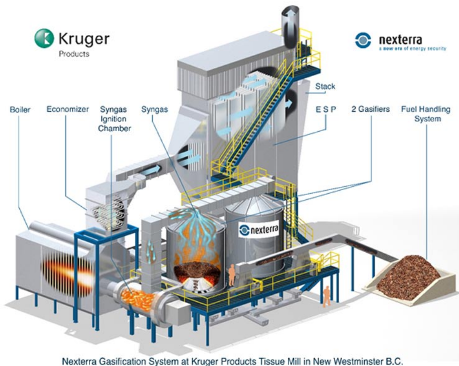
Nexterra Gasification System at Kruger Products Tissue Mill in New Westminster B.C.
