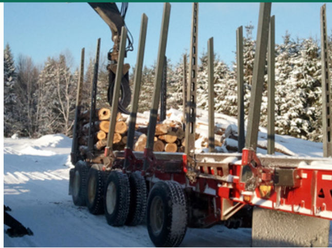
A part of the stakes and bunks is made of steel, and the rest of composite stakes and bunks. Spread out on the deck at strategic locations, they allow for the evaluation of their resistance to strain and impacts.
